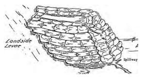
**Figure D.8** Sketch of ring levee tied to a levee slope, with spillway. Construction against the levee slope results in a U-shaped sandbag "chimney."
