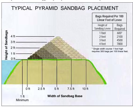
Figure D.4 Pyramid sandbag placement.
